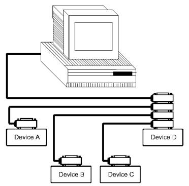
Figure 6-4 Typical GPIB System Interconnection for 4-piggyback Connector
