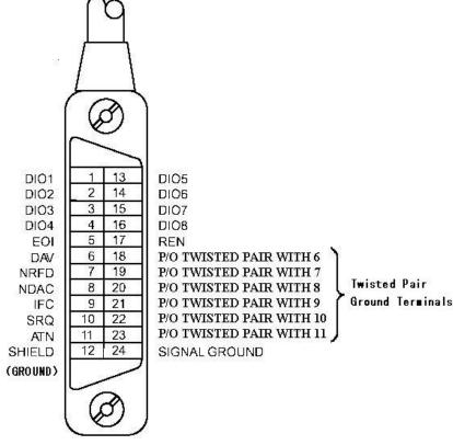
Figure 6-2 GPIB Connector/Pin Structure
