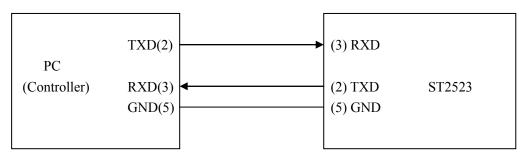
Figure 6-1 Connection of the instrument with a PC
